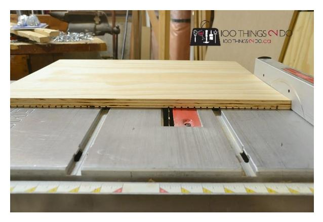
This may seem tedious, but you can notch one side, turn the board around and notch the other end without moving your guide rail - so two cuts from each measurement. To notch my entire back it took 15 minutes, and that's with taking photos as well.
