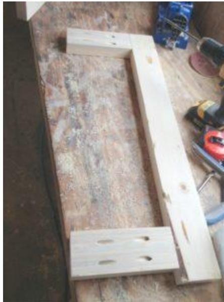
Before attaching the other 2x4 in the frame, I added a piece of 3/4" plywood to fit in the opening. It's best to measure and cut exactly to fit, but it should be 7" wide x 22 1/2" long.
