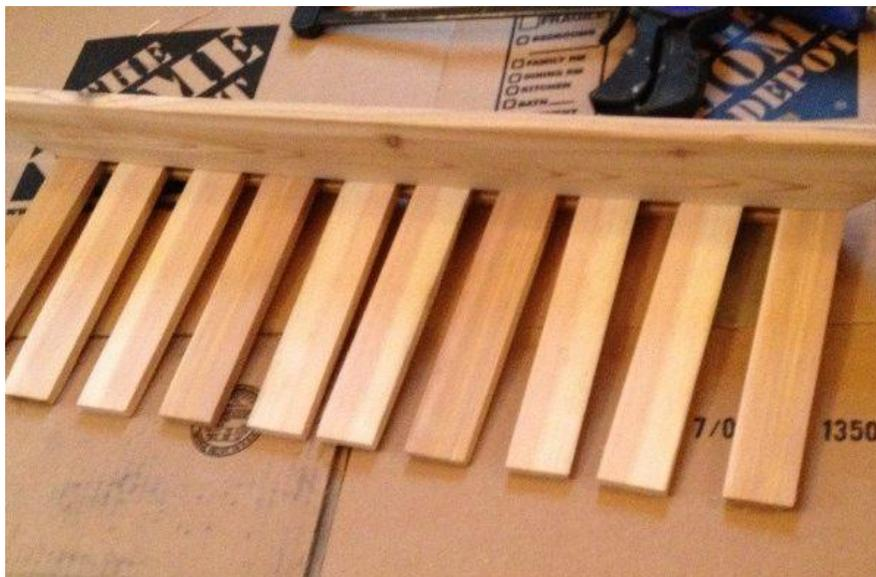
Chop the lattice pieces to your desired width, mine are 7 and 1/2 inches, for an overall caddy width of 8 inches. I used 10 pieces spaced 3/4 of an inch apart (this worked out nicely as I was able to use 3/4 MDF scraps for spacers).
