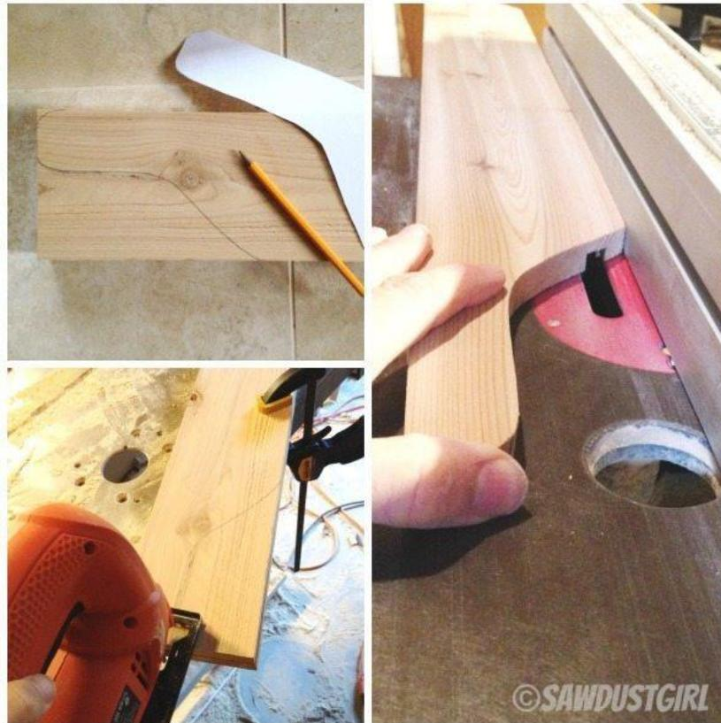
Print and cut out the handles template then transfer the shape to the ends of the pickets. Cut out the handles using a jigsaw or band saw. If one side is longer than the other (like mine) put the difference in the arms, so that the body remains even. Similar to building a drawer, cut a dado a half inch from the bottom on both sides. The dado needs to be 3/8 inch wide and 1/4 inch deep.
