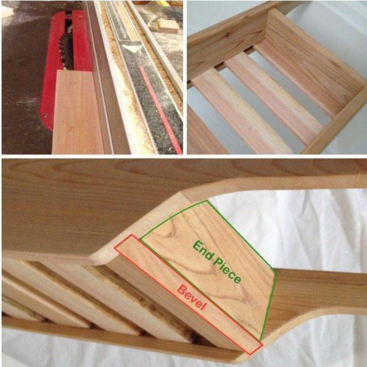
Use the table saw with the blade set to a 30 degree angle to bevel one edge of two lattice slats. These will be the outside ends of the caddy, the bevel fills the end of the dado flush and creates a more finished look than if the edges were left square. Next cut the end pieces from the scraps you saved earlier. These go on top of the outside slats. Mine are 7 inches wide by 2 1/2 inches tall, but adjust to your sizing.
