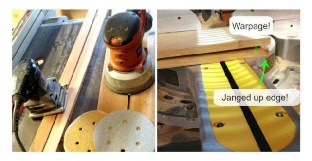
It is easier to do the major sanding before cutting this lumber. Start with a very rough grit, 36 or 50, to take off the scurf marks and really rough stuff. Then graduate up through the grits until they are nice and smooth. Cut all sides of the wood to give yourself clean edges and remove any loose knots or damaged wood.
