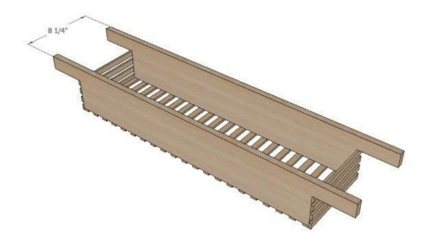
Attach the lattice slats with wood glue and staples. Start by attaching the 2 slats at each end and getting the caddy square. Then space the rest along the bottom 1/2" apart (or adjust to your measurements)
