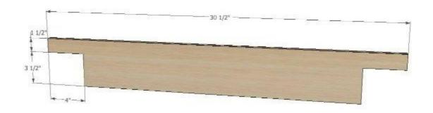
Rip two strips of the pickets 4" wide, then chop them to your desired length. Make a 4 inch by 3 1/2 inch cut out at each end of both pickets. These will form the arms and box for the caddy. Next cut 7" slats from the lattice, you will need 14 for plan dimensions, but adjust per your specs.
